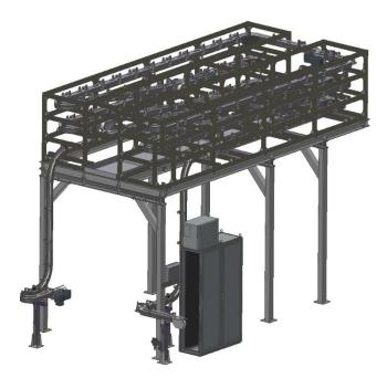
The advantage of the linear buffer system is that it can be positioned above existing equipment, thus creating new, previously unused production space.
